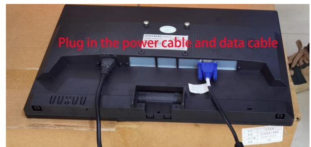
Fix the monitor's support, plug in the power cable and data cable in advance
