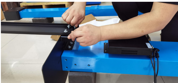
Fix the monitor's support, plug in the power cable and data cable in advance
