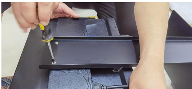
Fix the monitor on the support with 2 screws
